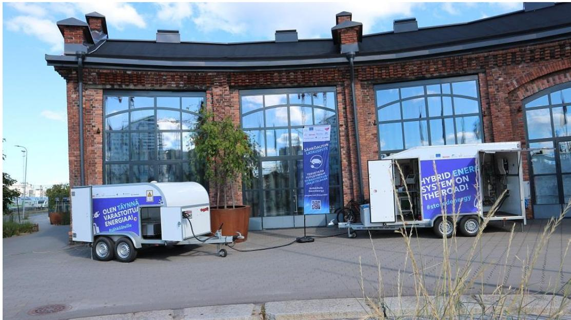
*Figure 1. Mobile hybrid energy system built in two trailers. The left trailer includes energy storage system, and the right one encloses power electronics system and high power charging station for electric vehicles. Technically versatile system offers excellent open innovation ecosystem for modern electric drives of smart energy transition. [3]*
